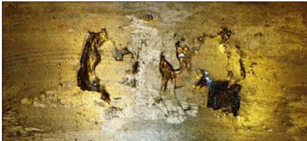
Figure 5. Photo of Wheel Tread Surface after Applying Etchant Martensite can be seen as the light gray areas between the spalls.
