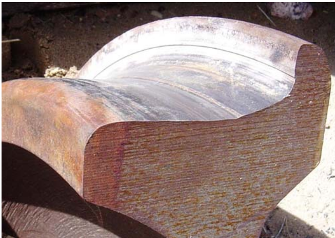
Figure 2. Cross Section from an Unusual VSR Wheel Showing Wear Groves in the Tread and Flange from Apparent Contact with the Brake Head
