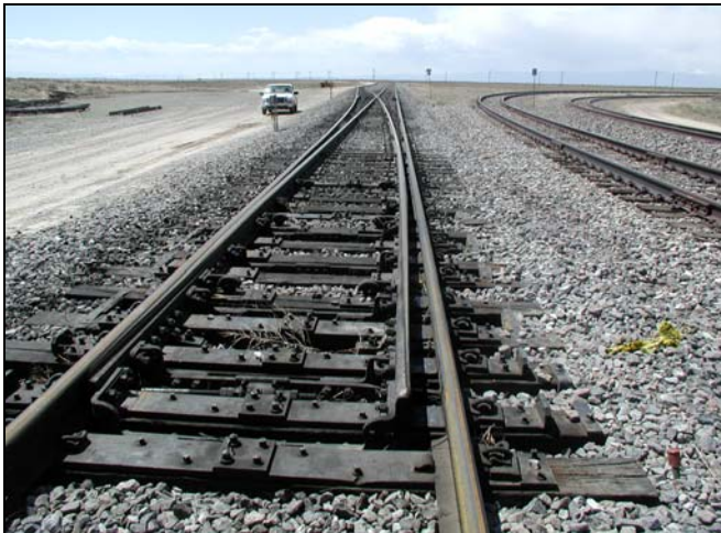
Figure 1. Typical Mainline Turnout
