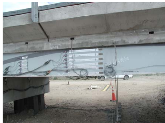
Figure 2. Gages for Measurement of Web Strains
