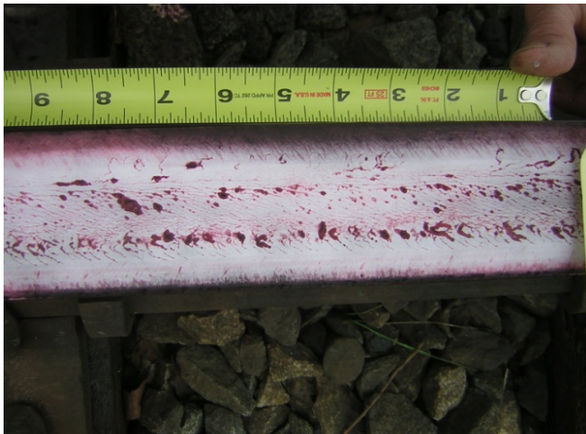
Figure 7. Low Rail of Curve S in the TOR-treated Zone at Site 3 Start of Test April 2006
