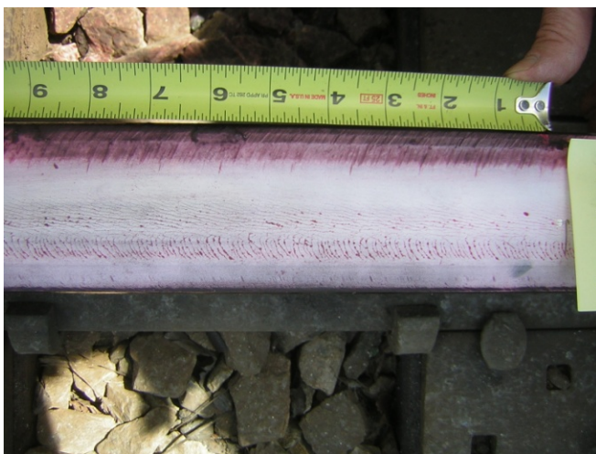
Figure 9. Low Rail of Curve D in the non-TOR Treated Zone at Site 5. Start of Test April 2006
