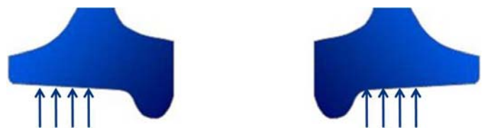
Figure 2. Wheel/Rail Contact Conditions Resulting from Asymmetric Wheel Tread Wear
