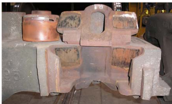
Figure 6. Indication of Uneven Wedge Pressures on the Truck Bolster
