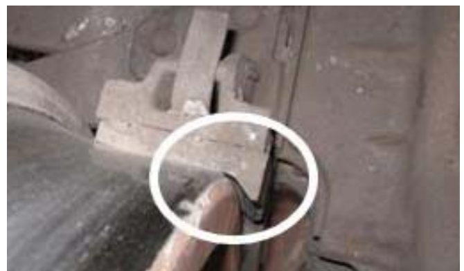
Figure 3. Overhanging Brake Shoe on Opposing Brake Beam/Wheel
