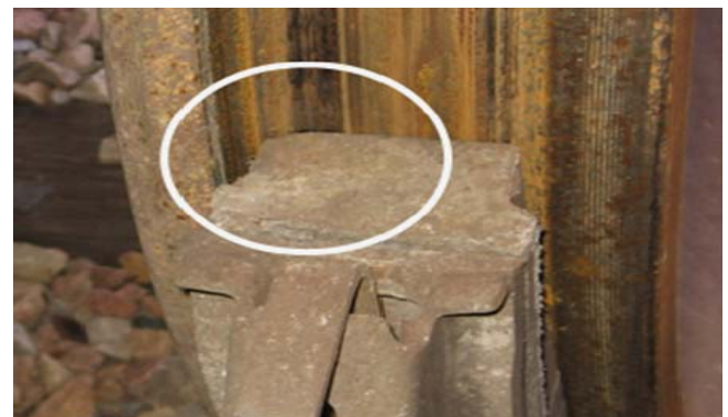
Figure 2. Overriding Brake Shoe Pressing against Worn Flange
