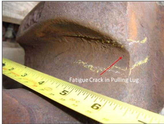
Figure 10. Fatigue Crack on Knuckle Pulling Lug
