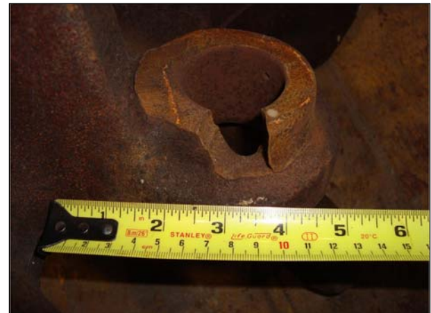
Figure 7. Coupler Pin Hole Defect
