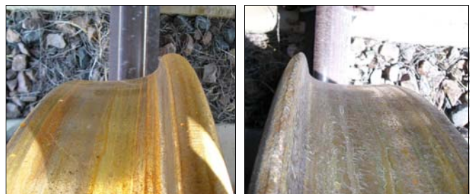
Figure 5. Articulated Car — Asymmetric Flange Wear on the Wheels of Axle Z
