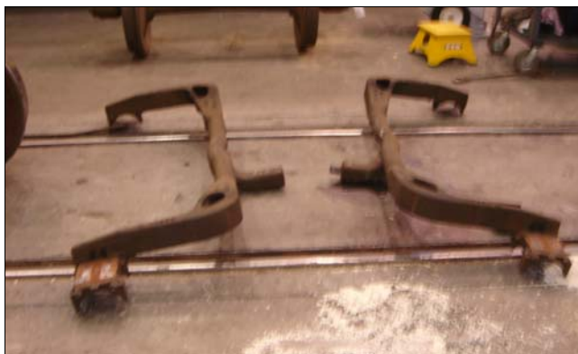
Figure 3. Autorack — Disassembled AR1 Steering Arms with Bearing Adapters Bolted in Place
