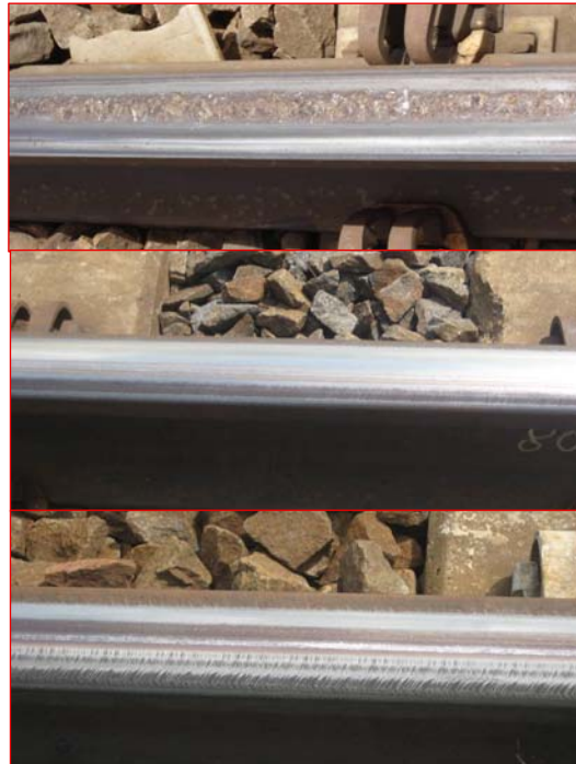
Figure 1. Rail Surface Conditions at 250 MGT (top – without TOR friction control or preventive grinding, middle – with TOR friction control, bottom – with preventive grinding)
