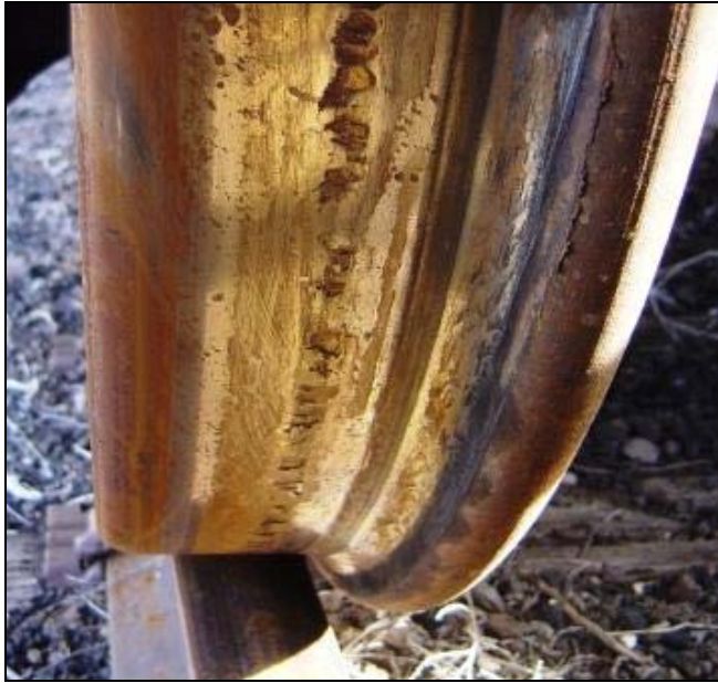
Figure 1. Wheel with Spalls
