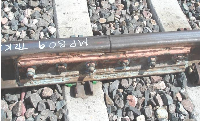
Figure 3. Conventional IJ with Kevlar Insulators in Track Removed after 1,000 MGT
