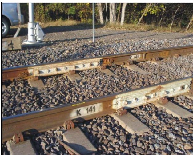
Figure 7: Side by Side IJ Evaluation of a Conventional IJ, and an IJ with Improved Surface Treatment and Durable Adhesive
