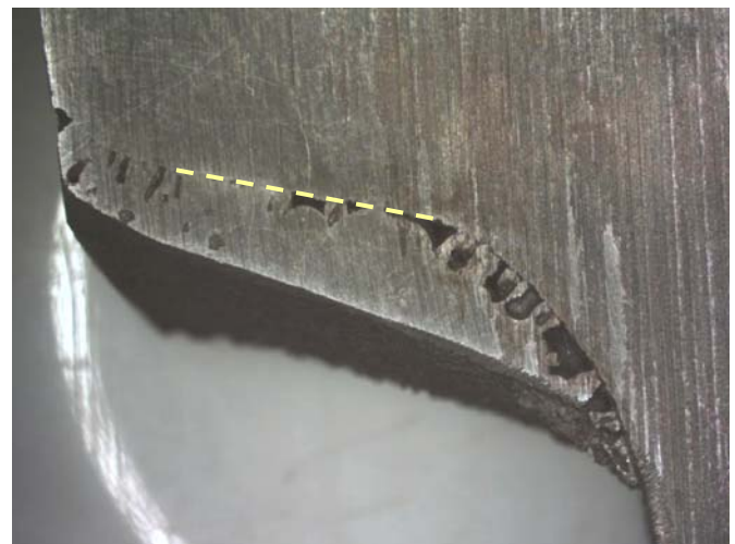
Figure 2. Transverse Cut of an OW-1 Weld showing Porosity in a Cold Lap under Railhead. Dashed line indicates location of bottom of railhead.
