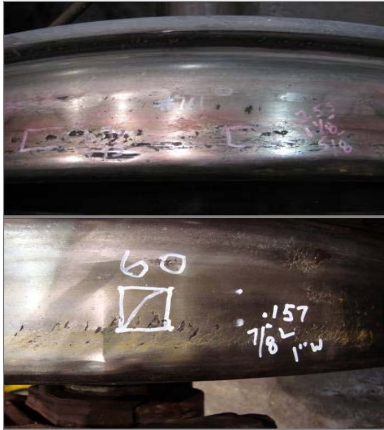
Figure 2. Typical Tread Shell Defects
