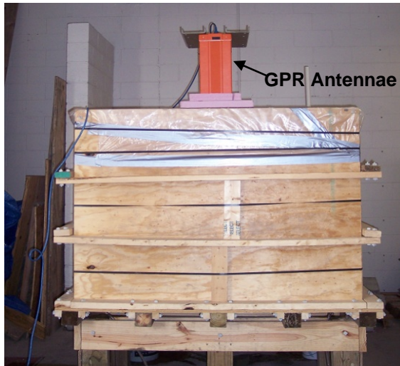
Figure 2. Wooden Box and 2 GHz Antennae Used for Ballast Testing
