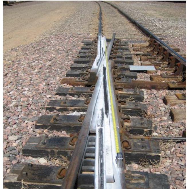
Figure 2. VAE Nortrak Jump Frog in Test at FAST
