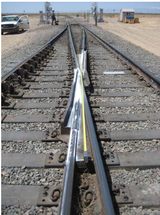
Figure 1. Progress Rail Lift Frog in Test at FAST
