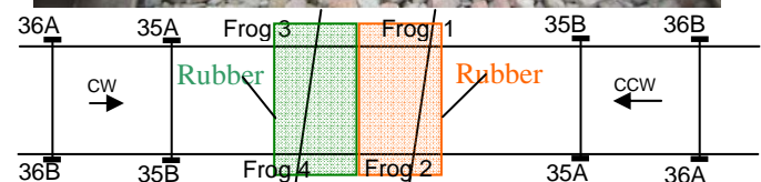
Figure 1. FAST Crossing Diamond and Layouts of IWS and Rail-seats
