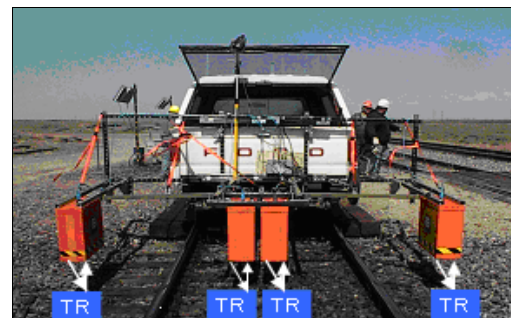
Figure 2. GPR Equipment Using Multiple 2 GHz Antennae
