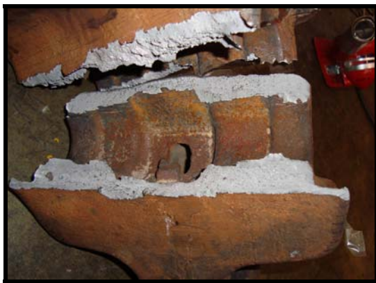
Figure 3. Knuckle Fracture Surface
