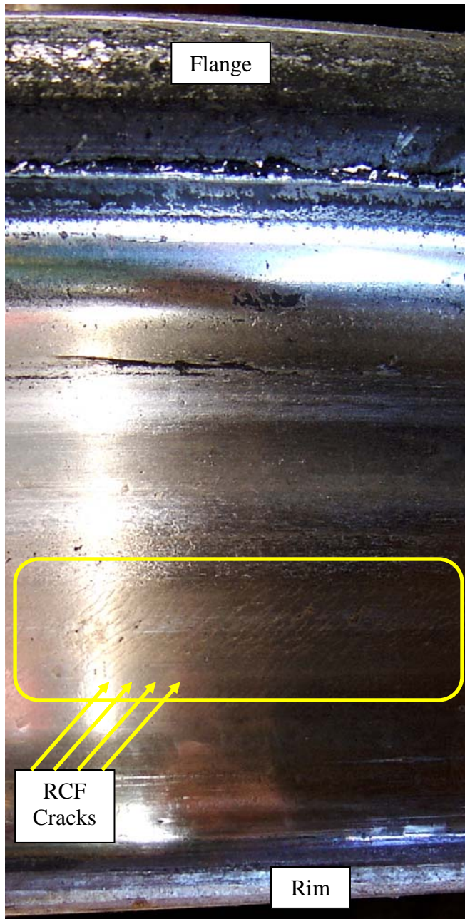
Figure 1. Example of RCF Cracks that were Too Shallow to Produce a Visible Result with Dye Penetrant Applied
