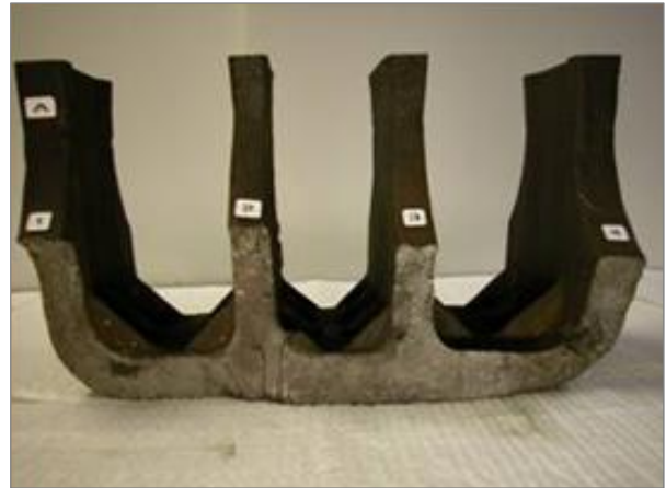
Figure 6. Fracture Surface of Failed Bolster
