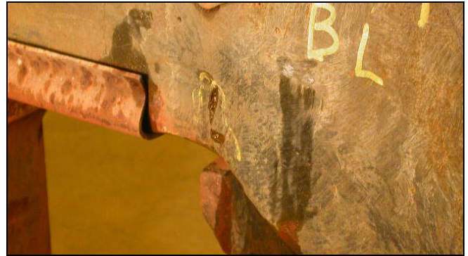
Figure 4. Defect Identified using Alcohol Wipe Inspection
