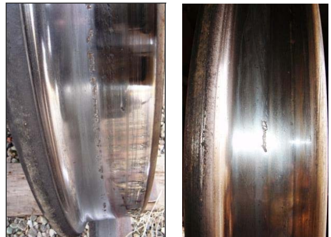
Figure 6. Minor Wheel Shelling was observed on Two Wheels
