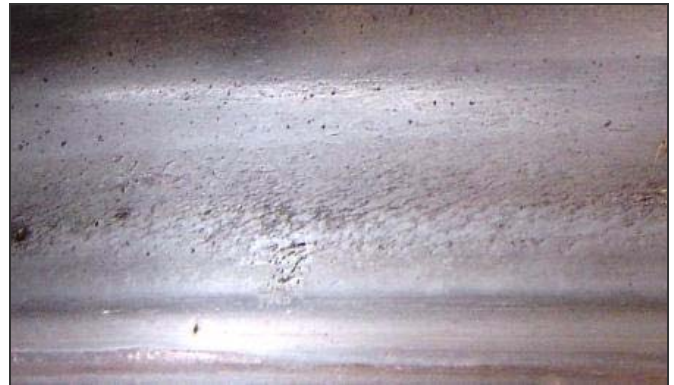
Figure 5. RCF Cracks were observed on 15 of 48 Wheels
