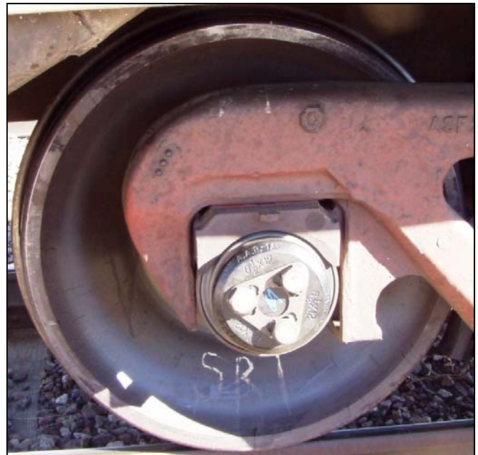
Figure 2. High Temperatures have Blued this Wheel Plate during the Drag Brake Test
