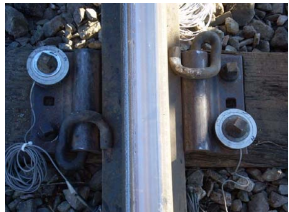
Figure 2: Top View of Pandrol Plate, Showing Measuring Load Washers
