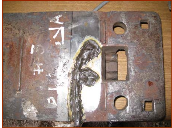
Figure 1: Bottom View of NorFast Plate, Showing Strain Gages
