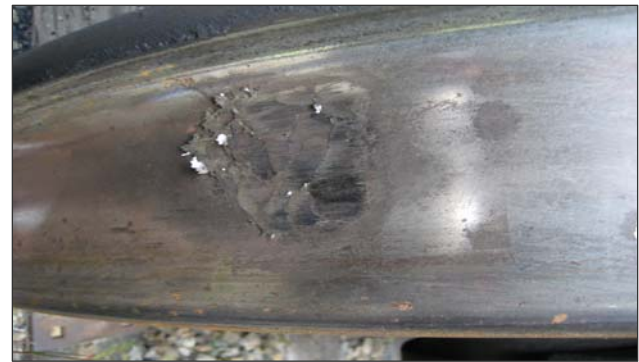
Figure 12. A Sizeable Wheel Flat
