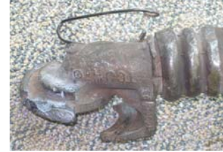
Figure 5. Hose Coupling showing Multiple Contacts
