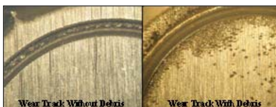
Figure 5. Micrographs of Wear Tracks with and without Debris
