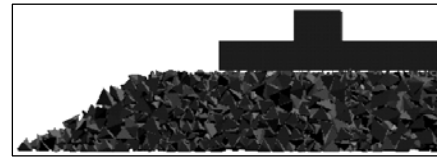
Figure 5. Half-tie Ballast Section — Profile View
