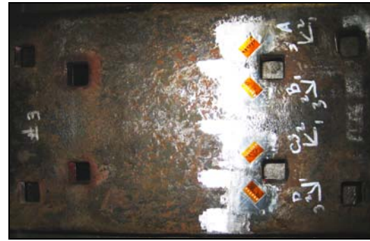
Figure 4. Strain Gage Locations on Tie Plate
