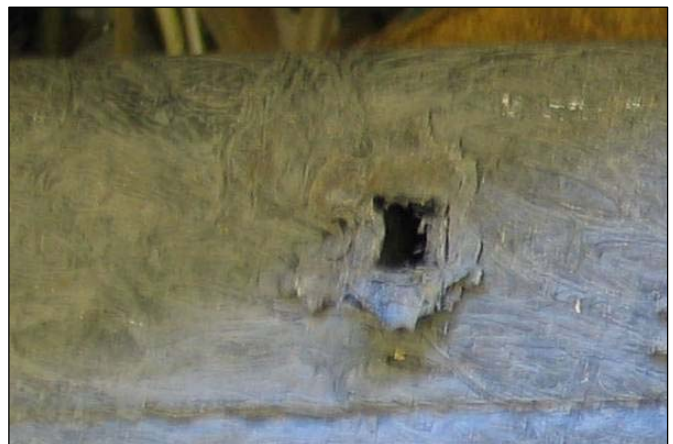
Figure 4. Plastic Extruded from a Cut Spike Hole
