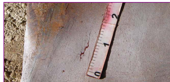
Figure 8. Tear on Transition Radius
