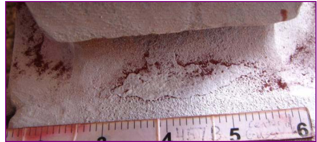
Figure 10. Scab on Pedestal Radius
