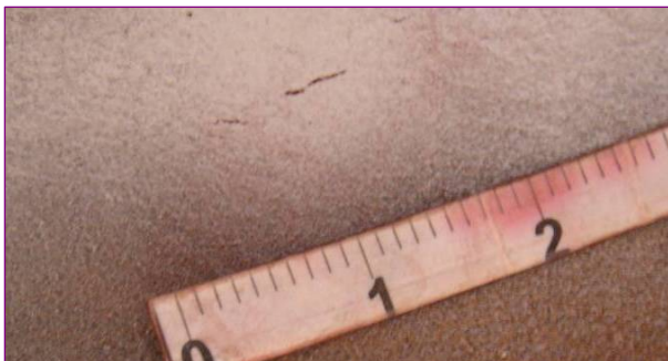
Figure 9. Tear on Spring Seat Radius
