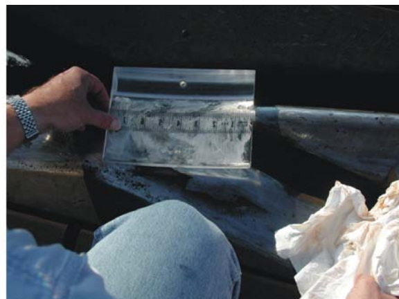
Figure 7. Flangeway Effective Gap Gage
