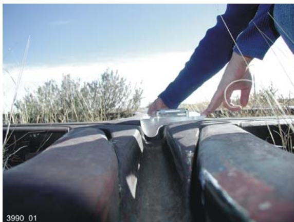
Figure 7. Flangeway Effective Gap Gage
