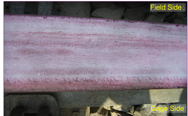
Figure 6b. Pre-Grinding, Optimized Gage Face Lubrication Only (Low Rail — Curve R, Site 1L)
