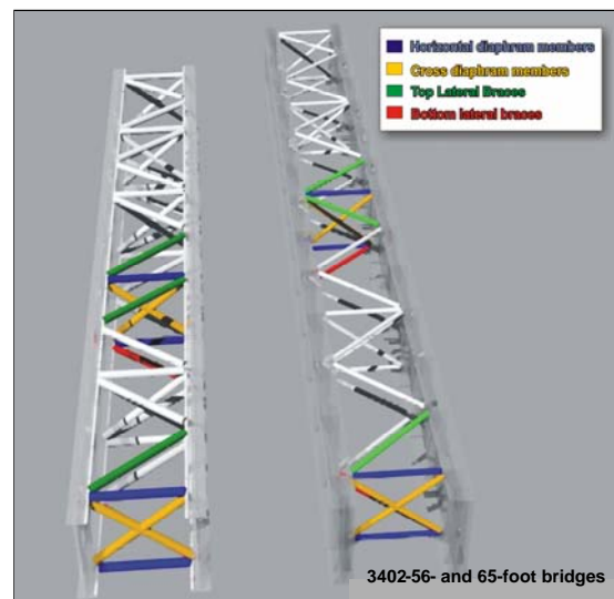
Figure 1. Strain Gaged Members of Bridge Spans
