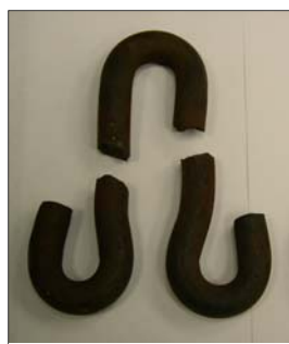
Figure 9. Parts of NorFast Rail Clips Fractured at 70 MGT
