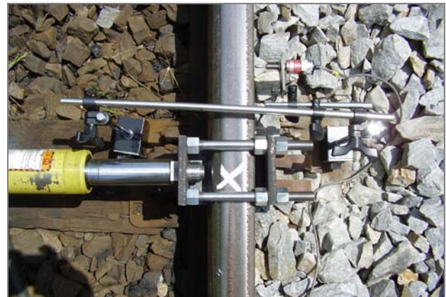
Figure 6. TPCI's Rail Rollover Restraint Fixture
