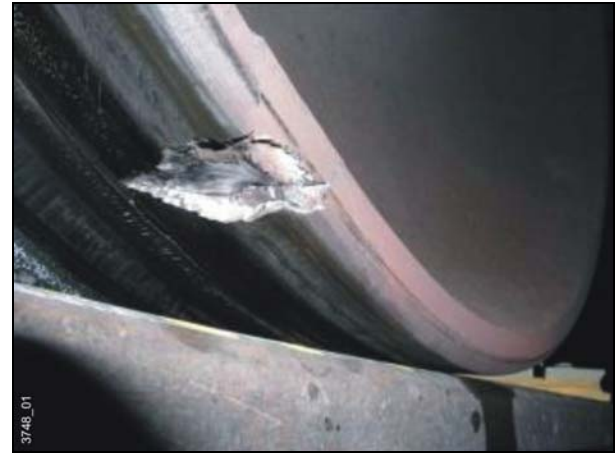
Figure 1. Shattered Rim Crack
