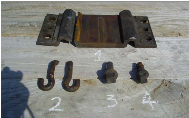
Figure 1. Component Failure under HAL Traffic (1) Pandrol 16-in. rolled steel tie plate (2) NorFast rail clip (3) LB&N High Strength Screw Spike (4) No. 5760 Screw Spike
