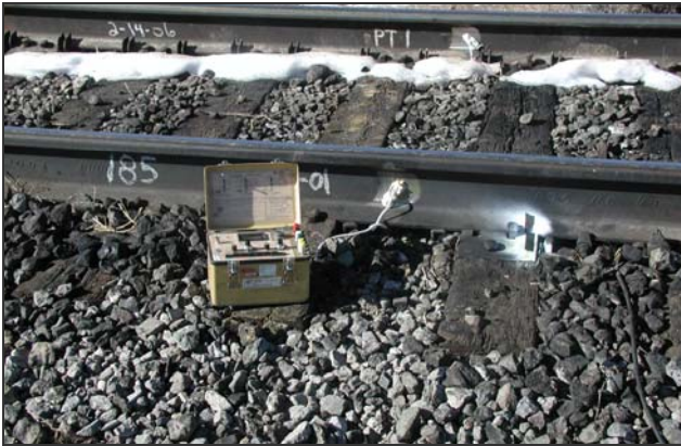
Figure 1. Rail Force Measurement Circuit
