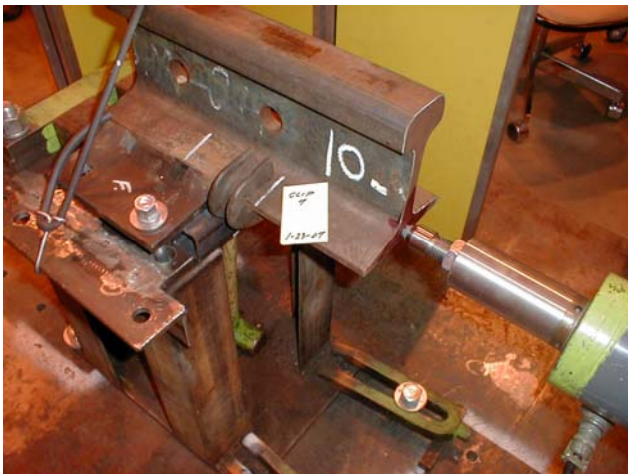
Figure 2. Rail Anchor Test Setup
