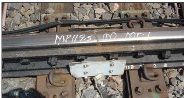
Figure 2. Wrap-Around Bars in Revenue Service Testing
