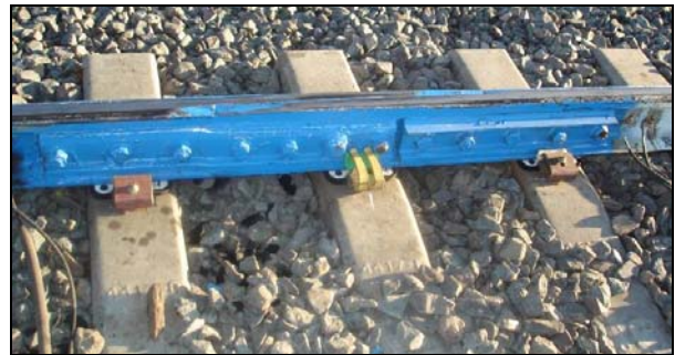
Figure 4. Taper-Cut IJ in Revenue Service Testing
