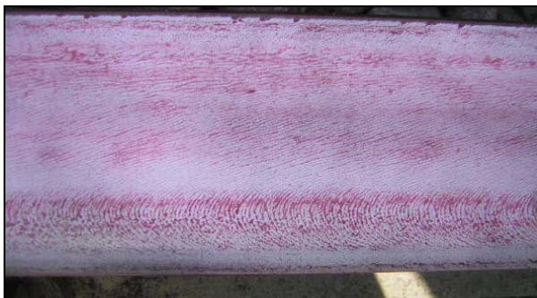
Figure 5b. Zone 1, Typical Low Rail after 95 MGT of Traffic
