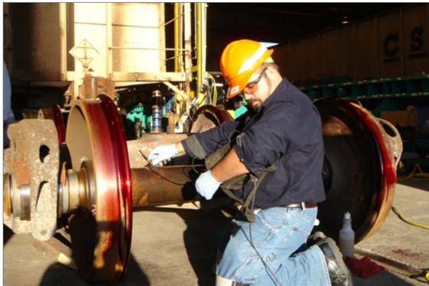
Figure 2. Truck and Wheel Inspections at CSX Avon, Indiana, Shop
