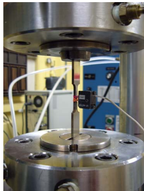
Figure 2. Weld Specimen in Test with Extensometer Attached
