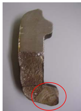
Figure 3. Joint Bar with Fatigue Crack. Removed after 75 MGT
