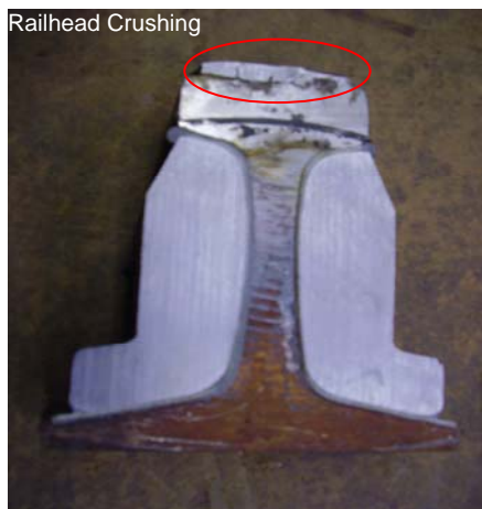
Figure 2a. Railhead Crushing, Prototype Removed after 300 MGT
