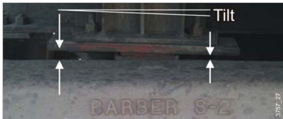
Figure 2. Tilted Body Side Bearing Wear Plate
