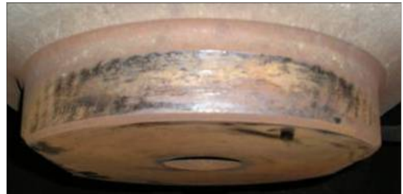
Figure 5. Chatter on Side Wall of Center Plate
