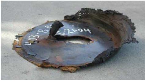
Figure 7. Flow or Extrusion of Polymer Center Plate Liner
