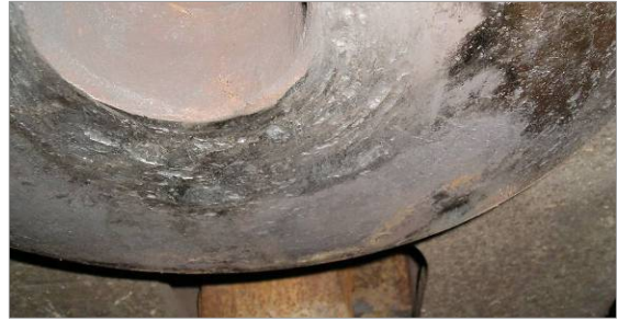
Figure 4. Galling of Center Plate
