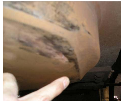
Figure 6. Material Flow on Chamfered Edge of Center Plate
