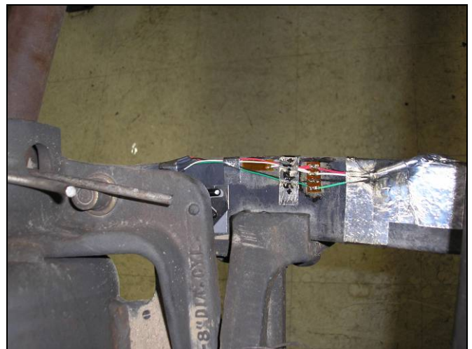
Figure 2. Strain Gage on the Compression Member of the Brake Beam
