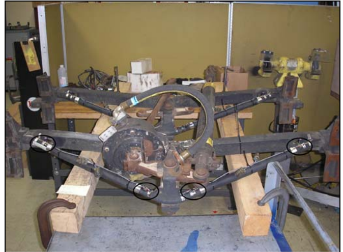
Figure 1. Strain Gages on the Tension Member of the Brake Beam
