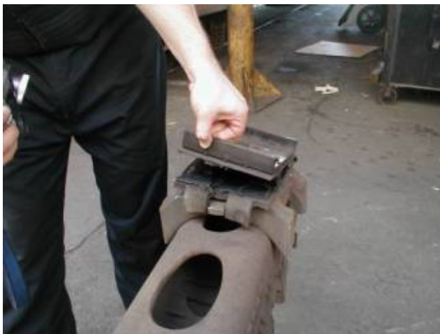
Figure 9. Failed Primary Pad
