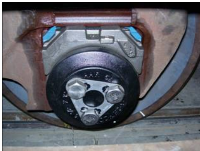
Figure 1. Elastomeric Pedestal Pad in SSRC Suspension
