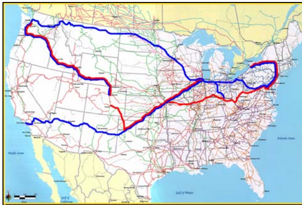
Figure 4. Travel Route of the Test Car, Blue = Loaded Route, Red = Unloaded Route
