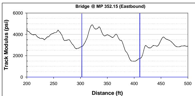
Figure 2. Track Modulus Test Result at MP 352.15
