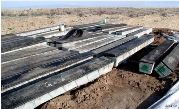
Figure 2a. Concrete Ties with Rubber Pads. Iteration 1, Pads Glued to Concrete Tie Bottoms at Site
