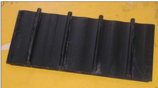
Figure 2b. Concrete Ties with Rubber Pads. Iteration 2, Pad Grooves Bonded Into Concrete Ties at Plant
